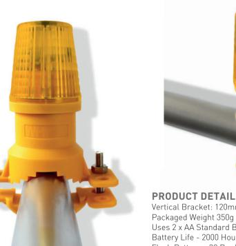
Vertical Bracket: 120mm x 155mm x 65mm Packaged Weight 350g Uses 2 x AA Standard Batteries (not included) Battery Life - 2000 Hours Flashing Flash Pattern - 30 Per Minute, (single flash) Duration of Flash 200 Milli seconds
